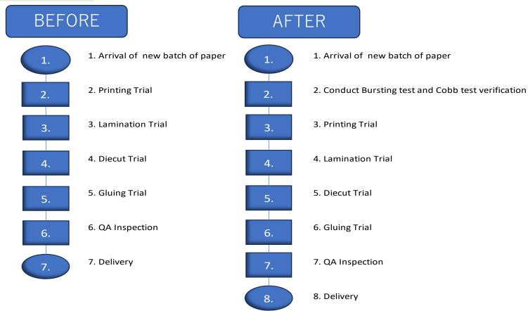
Invest COBB Test machine for ONSITE testing.
